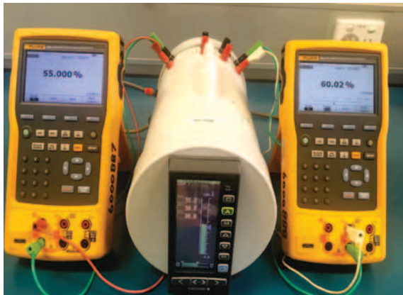
Proportional band set to 50% therefore a controller gain of two. A 5% input change causes a 10% output change.
